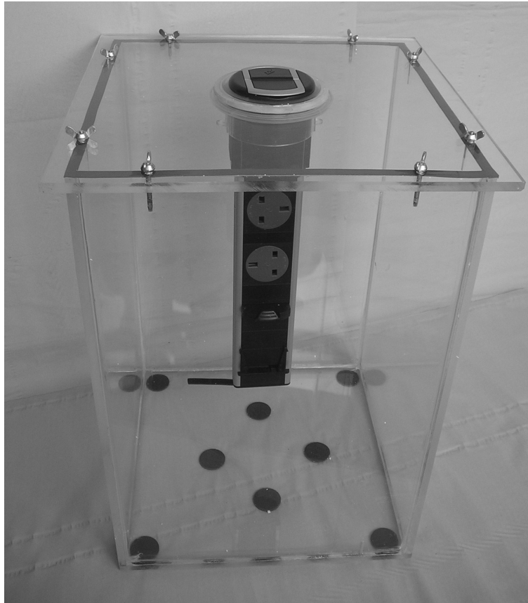
Power dock (domestic) fitted to the test enclosure supplied by the client
